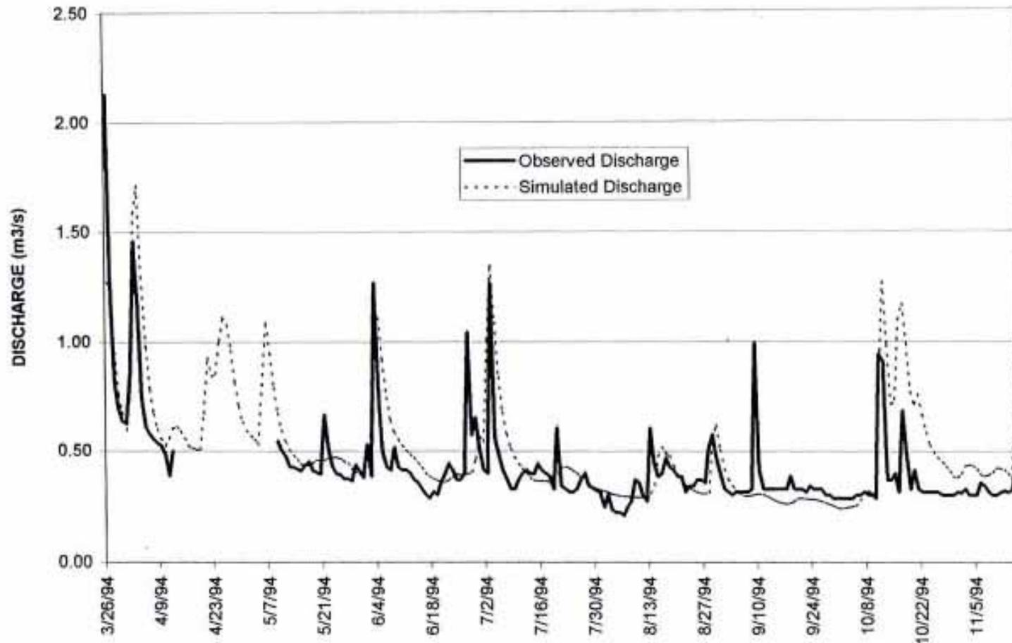
**Table 3.1.7 : Simulated Daily Streamflow Data at Temporary Dam for March - November 1994 (m3/s)**
