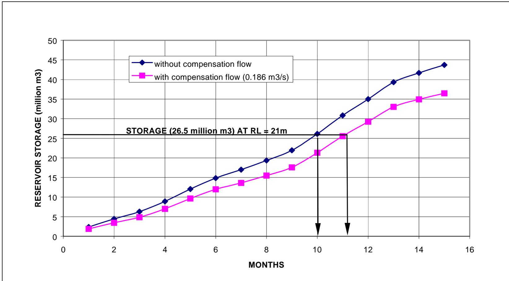
**Figure 3.1.9 Predicted Filling Times for Putrajaya Lake with and without Compensation Flow at 90% Probability (1 in 10 year dry minimum flow)**
