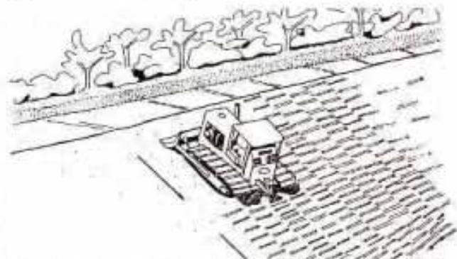
Figure 10.3 Preferred alignment of dozer track mark
