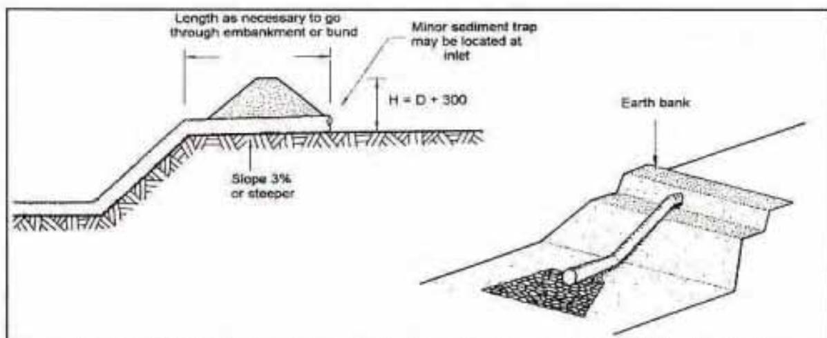
Figure 10.8 - Piping runoff over embankment (ref. Inst. of Eng., Australia, 1996)
