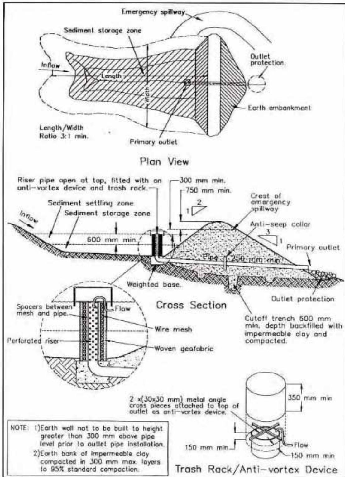
Figure 10.9 - Typical layout of a sedimentation basin (ref. NSW EPA, 1996)
