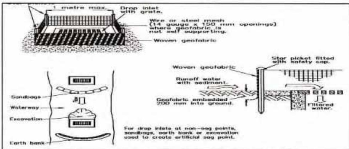
Figure 10.6 Location and installation of geofabric filters (ref. Inst. Engrs, Aust, 1996)
